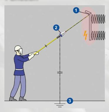
The voltage tester identifies whether there is operating voltage on a system part.
